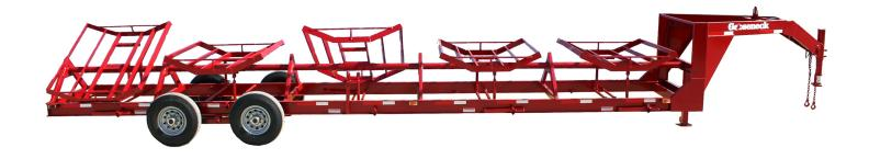
Our Haymaster trailer features a dual tilting mechanism that allows loading and unloading from either the left or the right. From feeding to hauling, we have you covered on both sides.
